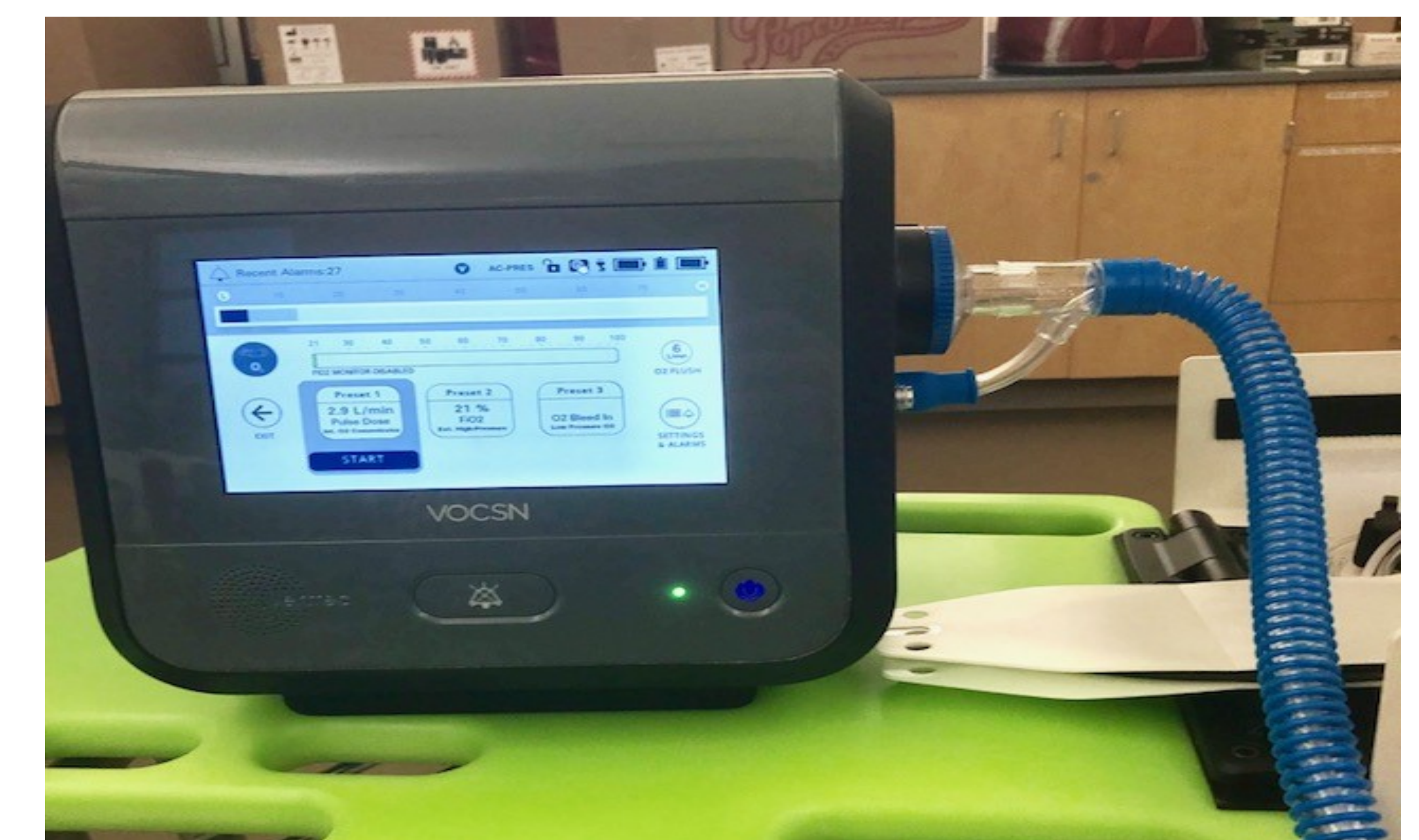
Figure 1. The VOCSN ventilator (Ventec Life Systems, Bothell, WA) provides both pulse dose internal concentrator (PDIC) and external concentrator (EC).
